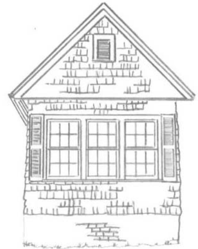
Original wood siding, wood shingles and original asbestos or masonite surfaces should be preserved and maintained.
